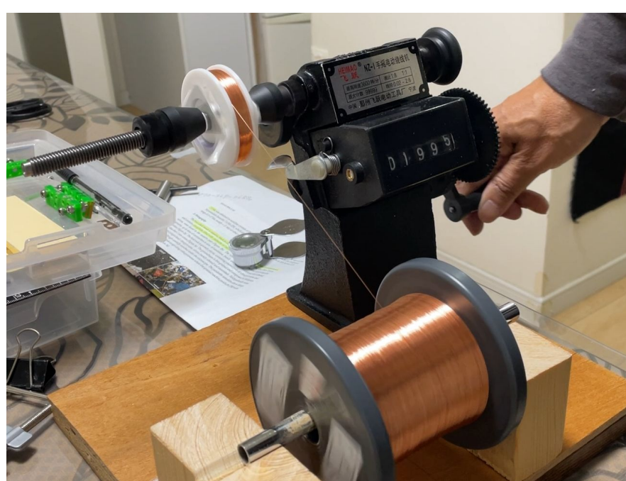
Fig.2 Hand coil winder with counter. Now 0.25mm urethane coil is winding
