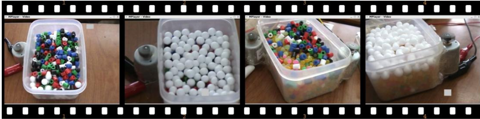
Fig13. Mixture of plastic balls with vibrate-motor mimic ground liquidizing.
