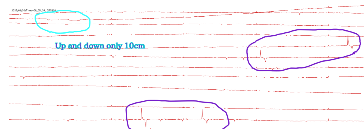
Fig.4 Dairy noise of door opens and closes with up-down sensor movement
