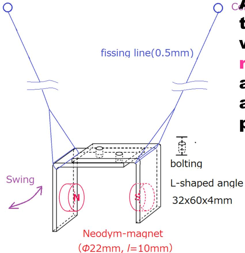
A magnetic circuit made of two L shaped steel plates with two columnar neodymium magnets forms a U-shaped bipolar magnet as a whole, also become a pendulum's weight.
