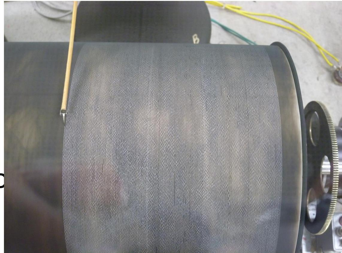
**Omori type mechanical seismograph
