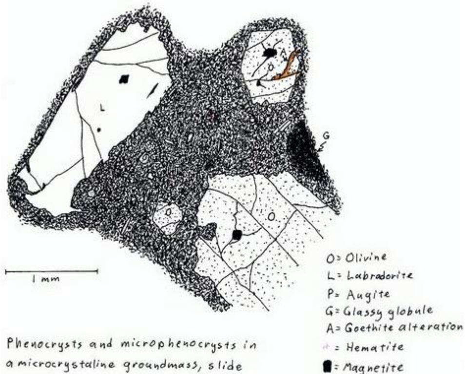
Phenocrysts and microphenocrysts in a microcrystalline groundmass, slide HW-8A.
