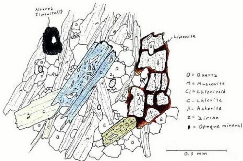
Typical Mineral relations. Note alteration of opaque mineral (ilmenite?) to a nearly opaque pseudomorph (leucoshe?), and ankerite to limonite. Also note sharp, unreacting contact between chloritoid and chlorite.
