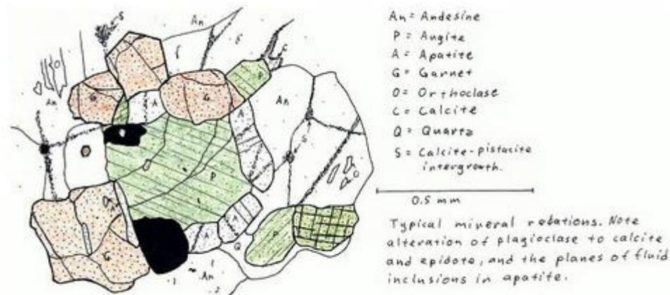
Typical mineral relations. Note alteration of plagioclase to calcite and epidote, and the planes of fluid inclusions in apatite.
