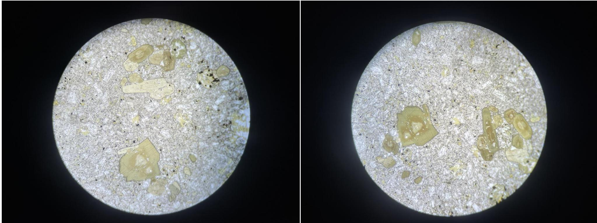
Refraction index (Open polar): **Olivine**, Pyroxene,
